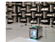
ISO 3744 acoustic test
