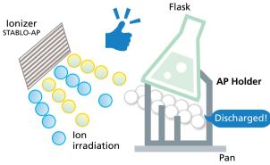
Using the AP Holder to separate the flask from the pan, the ions supplied by the ionizer reach the locations where there is static charge on the bottom of the flask. This improves the neutralization effect and results in a stable weight value.
