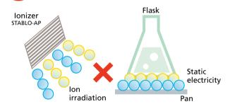
lons emitted from the ionizer cannot reach the bottom of the flask, so removal of static charge from the bottom of the flask is insufficient. Therefore, Coulomb forces act between the surrounding metal parts and the windshield door, which affects the weight value.
