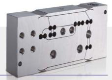
Shimadzu introduced one-piece force cell technology for precision balances in 1989. Today's UniBloc is created by high-precision electric discharge wire processing applied to a block of aluminum alloy, and replaces the conventional electro-magnetic balance sensor assembly. UniBloc's compact, uniform structure ensures stable temperature characteristics, excellent response time and stable corner-load performance.
