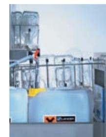
**Two peristaltic pumps** automatically dose the liquid detergents and neutralisers during the cycle. The chemical intake time is preset, and user adjustable. Chemical products are thus maximized, and the handling dangers due to the use of powder detergents disappears. An **automatic liquid level detector** is provided as standard for two chemical containers.
