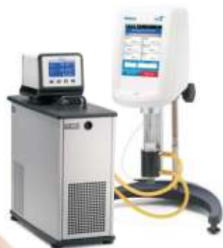
Water-Refrigerated-Circulating Bath (to maintain temp. @ 25°C)
