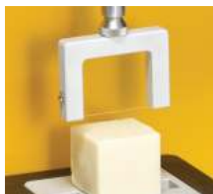
TA-WSP Wire Shear Plate cuts through the sample. Good for products with significant stickiness like cheese and butter. Fixture Base Table required.
