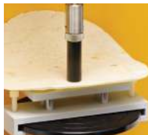
TA-JPA Junior Punch Fixture is for punching through flat samples; 12.7mm max. diameter probe. Hole in fixture is 14mm. Rotary Base Table required.
