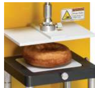
TA-CTP Compression Top Plate for applying uniform compression forces on samples up to 4x6 inches (10x15cm) Fixture Base Table required.
