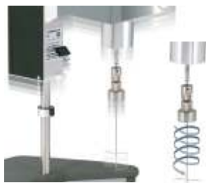
Helipath Stand (to measure viscosity of cream & paste)
