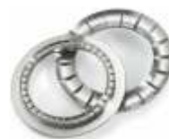
Close-up View of Wall Friction Lid for wall friction test and density test
