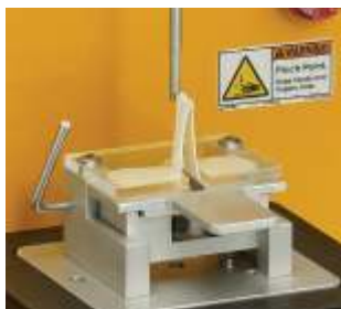
TA-KF Kieffer Dough and Gluten Estensibility Fixture quantifies maximum force and distance needed to break sample. Fixture Base Table required.
