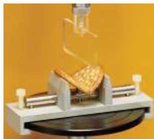
TA-JTPB Small scale version of Three Point Bend Fixture is used with TA7 blade from general probe kit. Rotary Base Table required.
