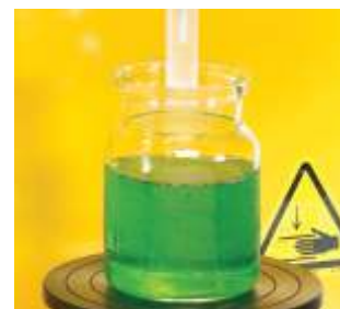
TA-10 GMIA & GME probe and spec Bloom bottle TA-GBB-2 sold in package of twelve bottles. Rotary Base Table required.
