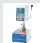
CAP 1000+ Cone/Plate • Single Shear Rate • Required for Paints and Coatings
