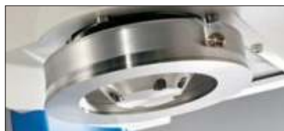
Close-up View of Wall Friction Lid for wall friction test and density test
