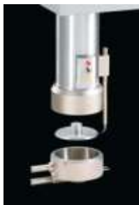
Wells Cone & Plate (to measure viscosity of sample volume as low as 2 ml)
